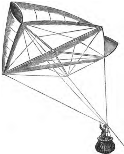
A KITE, composed of fabric strengthened by means of a net
